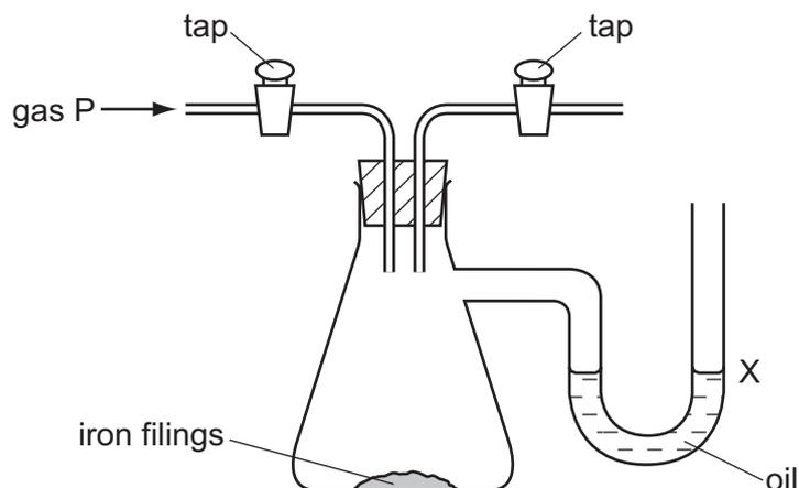
The flask is filled with gas P. The taps are closed and the apparatus is left for a week.
